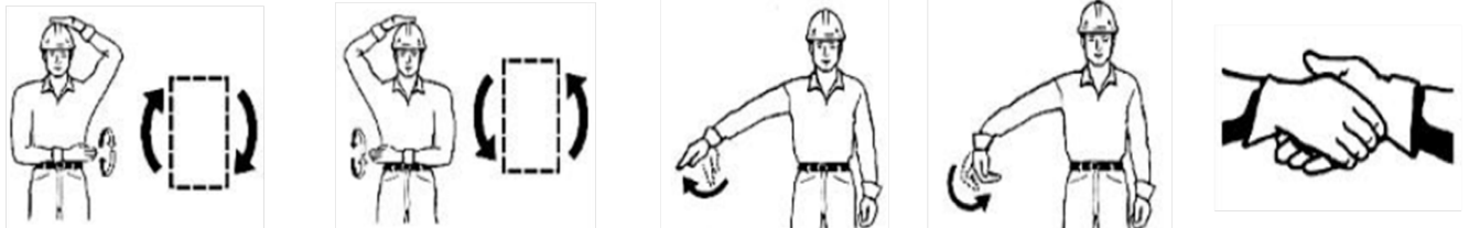
Counter Rotate Right Counter Rotate Left Open Bucket Close Bucket Dog Everything
