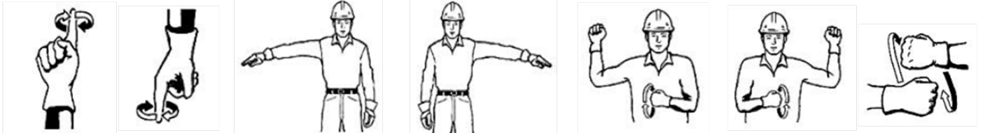
Load Up Load Down Swing Left Swing Right Turn Left Turn Right Travel
