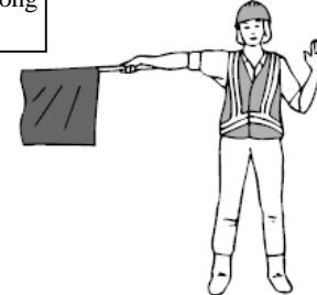
**Conclusion:** Hand signaling devices are an essential part of controlling traffic in temporary control zones. Flagmen should wear high-visibility clothing, stay off the roadway and out of the path of oncoming traffic, and use only the stop/slow paddle or red flags to direct traffic. Employers should train all flagmen in the proper signals used to control traffic. Always utilize these safety guidelines and have these signals posted wherever flagmen work.
