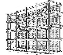
**Scaffold Toeboards:** A **scaffold platform** is a work surface raised above lower levels. A walkway is a portion of a scaffold platform used only for access, and not as a work level. All scaffold platforms must be planked between the front uprights and the guardrail supports. Toeboards are to be in place below the guardrails.
