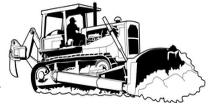
**Conclusion:** Because of the incredible power, sensitive steering, and the uncovered tracks which commonly throw mud, rocks, and debris, Bulldozers should not be operated in close proximity to unprotected personnel. If this is unavoidable, the machine should be operated at the slowest speed possible to perform the task with throttle control set to a lower setting than during normal operations. Follow these guidelines for safe Bulldozer operations.
