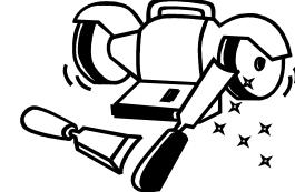
**Requirements for Machine Guarding of Grinders:** Guards must be made of steel or other material with adequate strength and must enclose the wheel sides. It is necessary to maintain clearance between the wheel side and the guard. This clearance should not exceed one-sixteenth inch.
