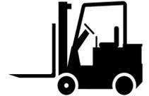
**Forklifts:** Do not allow anybody underneath raised forks, regardless of whether forks are loaded or empty. Handle only loads that are stable and safely arranged. Do not handle loads in excess of the forklifts capacity, or any attached component's rated capacity. Always place forks under the load as far as possible when lifting. Do not tilt the mast forward unless setting the load down. Use only compliant platforms to lift people.
