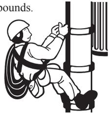
**Body belts** worn around the waist may be used in positioning device systems, but not in personal fall arrest systems.
