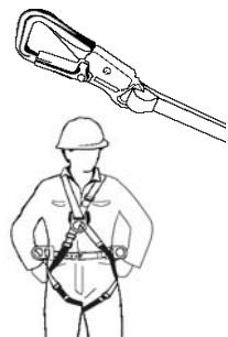
**Other hazards:** Fall protection is required for workers exposed to the hazard of falling into dangerous equipment or any other elevated ramp, runways, walkways, or working surfaces.
